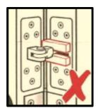
Installing the closer the wrong way will result in failure and is not covered by the manufactures warranty or guarantee.
