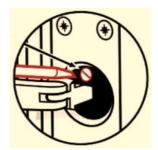
To safely hold the door in an open position where it is possible to fix the closer in place. The closer is suppled with a retaining plate. Care should be taken when inserting the closer to ensure the plate is accessible, but at no risk of being knocked off, as the force of the spring in the closer may cause injury.
