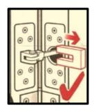
Remove the retaining plate. Ensure that it is kept in a safe place in case it is necessary to remove the closer from the door at any time in the future.
